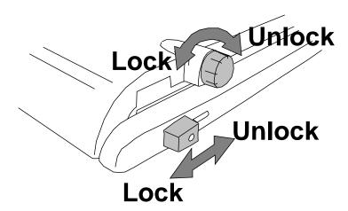
Release the brake on the reading table and pull the table out towards you. If you push the table back in again, you will see that the table locks home only when located centrally between its legs. Place some text on the table and you should see it on the screen.
