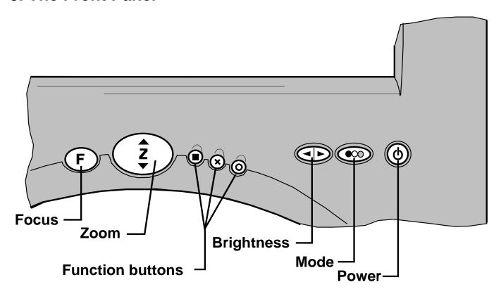
The front panel has eight buttons that control the various function of the Andromeda. Throughout this manual the buttons will be referred to with symbols. The exact function of each button may vary depending on the way the Andromeda is configured and its current mode of operation.
